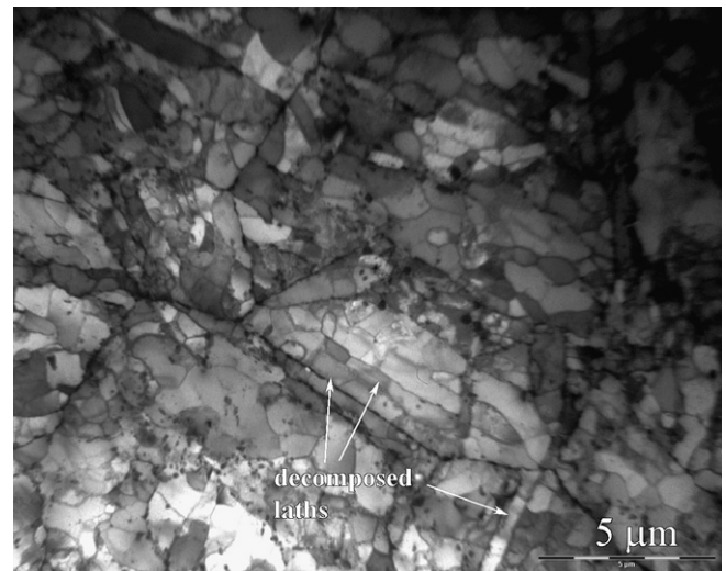
Fig. 6. Cell structure induced by the cyclic deformation in Eurofer 97, tested in air, at room temperature, at 0.8% total strain, for 7261 cycles.
